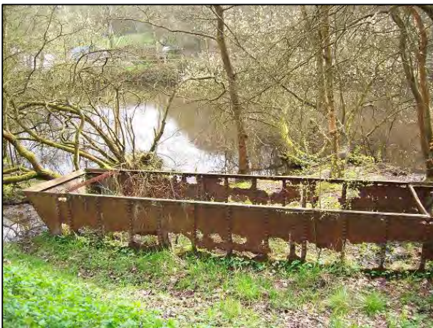
Canal Head with remains of horse drawn iron barge used to transport coal mined in Ernecroft Wood to the mills.
