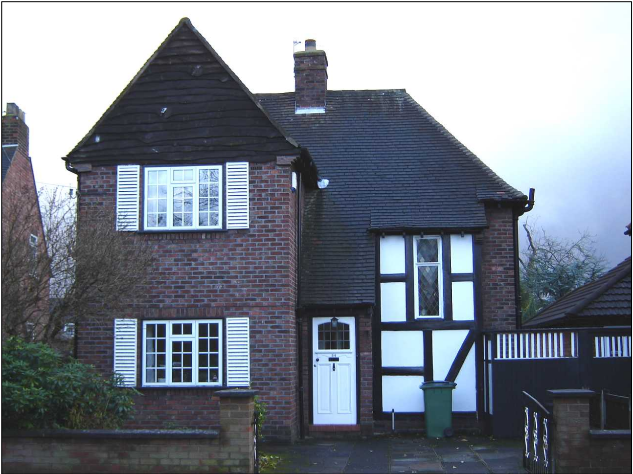
Cavendish Road. Interwar house with vernacular revival features in the tiled hipped roof, cat-slide porch, steep waney-boarded gable and half-timbering. The panelled door and leaded-glass staircase window are also original features.
